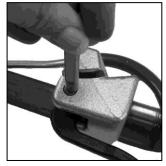
3. To replace Pin, Gripper Spring must be seated in Tension Screw hole. Align Gripper hole with Slide Block hole and insert Pin using a hammer.
