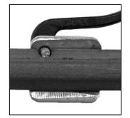
1. To remove Gripper, align Gripper Pin hole with notch in tool frame. Using a punch and hammer, punch Pin out of Slide Block.
