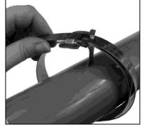
2. Insert band around workpiece again and through buckle. *Double wrapping develops much more radial compression than single wrapping.* Bend end of band under buckle.
