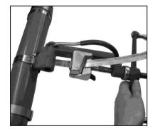
5. Roll tool over buckle, backing off with Tension Handle 1 -  $1\frac{1}{2}$  turns throughout entire rolling operation. Failure to back off tension with tension handle throughout roll-over may result in breaking the band. There is no loss of tension as band released is used up in this process.
