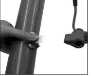
7. Remove tool, holding stub of band down.
