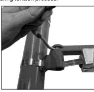
6. Rotate Cutting Handle forward to cut the band. When applying Giant Band clamps, prior to cutting off clamp, release Band Gripper and push Tool Nose away from buckle approx. ¼".
